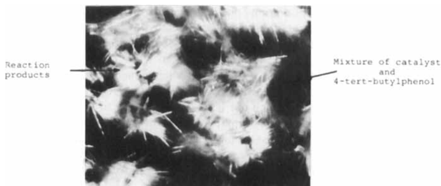
FIGURE 1 Hydrogenation of a polycrystalline 4- tert -butylphenol block in the presence of traces of catalyst.
